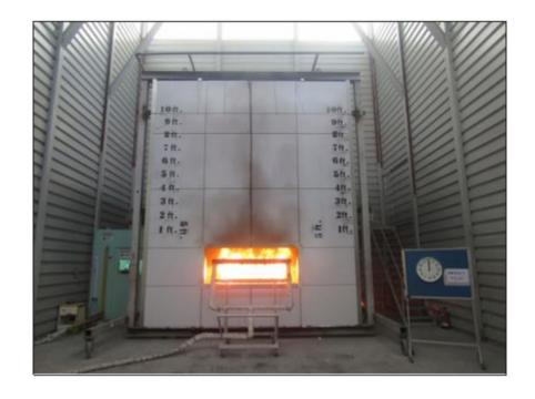
Fire propagation of an exterior non load bearing walls according to NFPA 285 (US standard mandatory e.g. in UAE)
