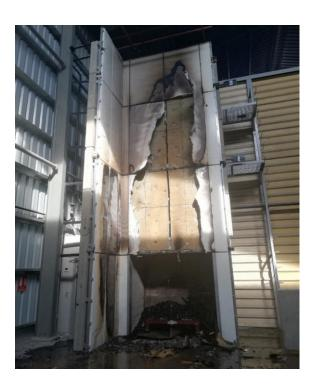
Fire propagation of an exterior non load bearing walls according to BS standards
